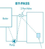
Wired in series so cylinder thermostat on demand will activate the boiler and <u>OPEN</u> the motorised valve (normally closed version)
