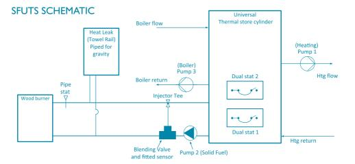
This schematic is for solid fuel pumped circulation. Note: A heat sink must be fitted
