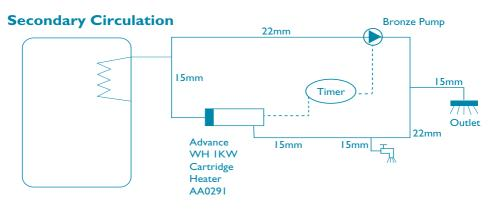
Set the WHI at  $45^{\circ}$ C to maintain temperature in the secondary loop without affecting the store temperature, costing just pennies per day.
