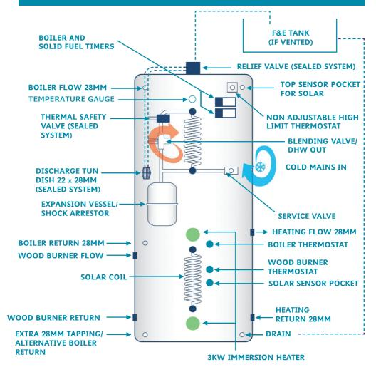
IMPORTANT: Gravity circulation must be achievable through the store from the woodburner. The store must be on the same level or higher - see diagram on page 6.
